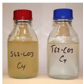
Figure 1: Example of water quality improvement between conventional valve (left) and Typhoon System (right)
